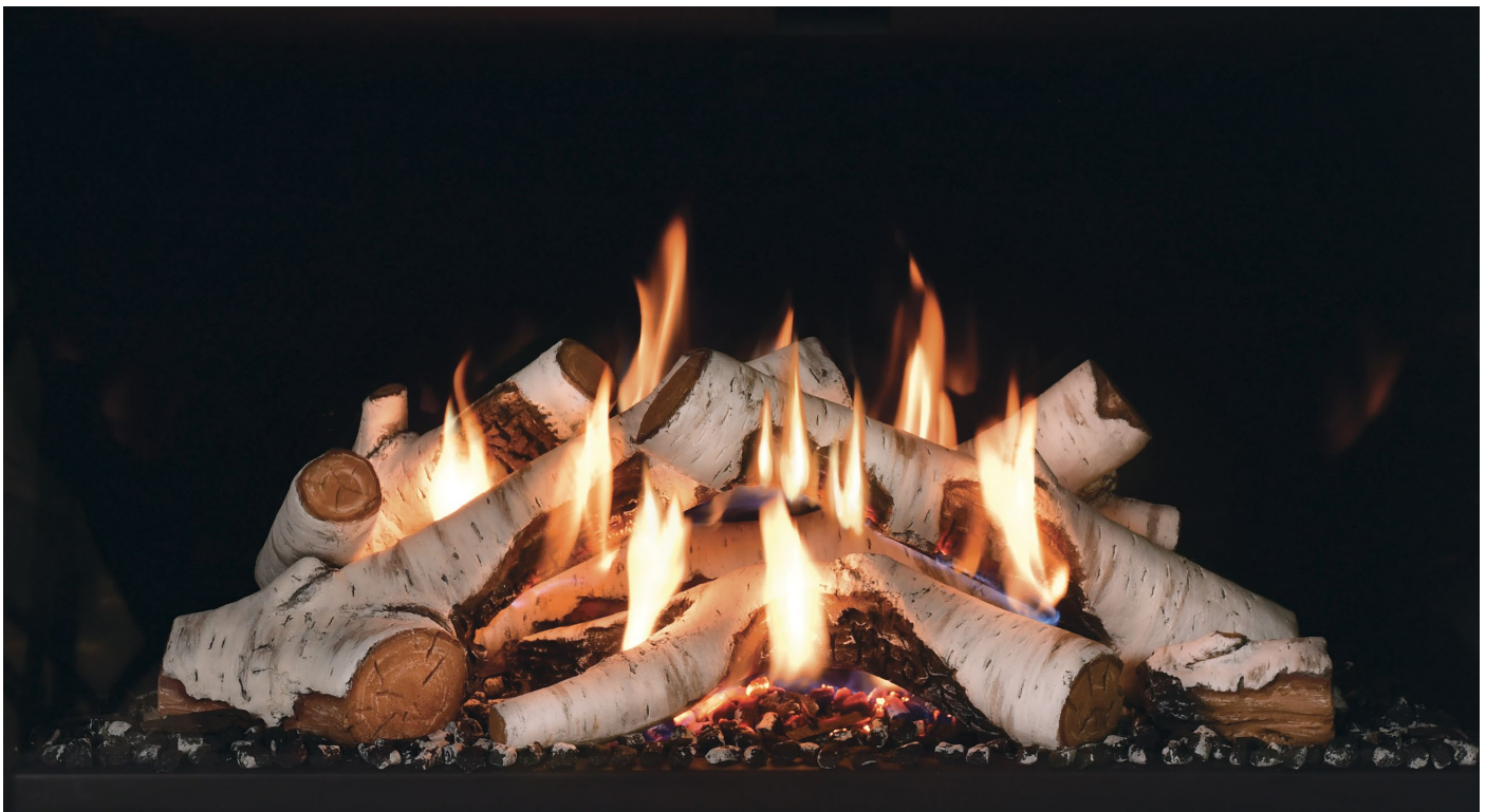
Figure 6-2 Burner Flame Heights: This image provides a visual reference for the burner flames burning at maximum height after the burners have been operating for 30 minutes or longer. A normal rear flame will be 1 to 2 inches above the rear log top edge. This, however, is dependent on the gas type, air shutter opening setting and vent system configuration. Actual flame heights can be slightly higher or lower when compared to this reference image.
